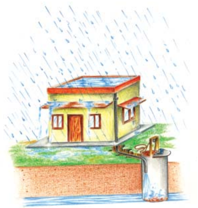
(b) Recharge through Abandoned Dugwell
