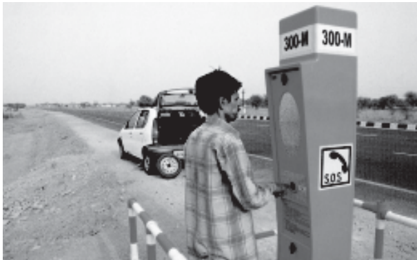
Fig.7.10 : Emergency call box on NH-8
